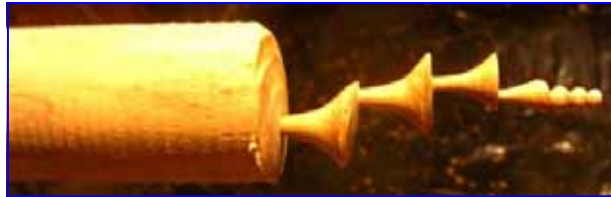
This and the next two pictures show how a piece might evolve by turning the chuck every so often to create off-balance work
