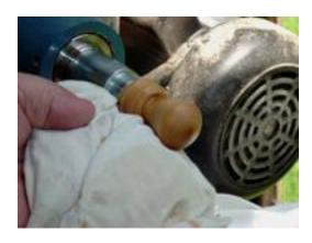
Apply your favorite finish. You can use a French Polish or some other finish. Here I used two coats of lacquer sanding sealer and one coat of Mylands Friction Polish. I sand with 400 grit between the coats of sanding sealer.
