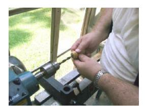
Apply yellow wood glue or CA glue on the dowel and press into the stopper.
