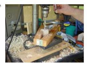
I use a 3/8 X 16 tap to tap the hole (this is for the chrome cone bottle stopper). On hardwood the treads made by the mandrel might not be long enough and it will leave a gap between the cone and the wood. It is almost impossible to get the cone up to the wood if the threads are not long enough so I use a tap to ensure that the threads are deep enough.
