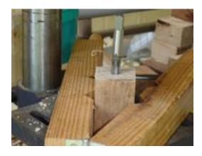
The block is mounted on the mandrel. The tail stock is brought up (using a small piece of wood so the indentation from the center is not in the stopper) to prevent it from turning in the mandrel if you get a catch. With a good catch it will come off the mandrel. You can remove the tail stock after the blank is round.
