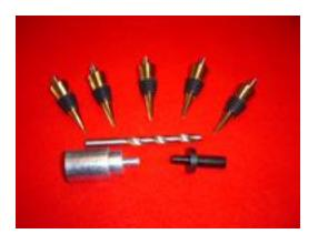
This is the Berea type bottle stoppers. They require a different mandrel that mounts in a drill chuck and it uses a 6 mm drill bit for the hole. You can purchase the mandrel and cones from Arizona Silhouette.
