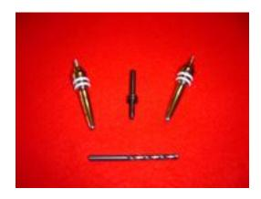
This e-book illustrates how to turn a chrome cone bottle stopper. Using similar techniques you can turn natural cork, silicon, or Berea type bottle stoppers. Drill a hole approximately 1" deep in the block using the supplied drill bit.
