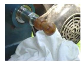
Remove the stopper from the mandrel. Remember to finish the bottom.
