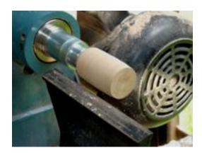
I start with a taper down to the mandrel. The diameter of the mandrel is the size of the chrome cone stoppers. This taper provides a transition from the cone to the wood.
