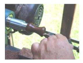
Apply thin CA glue around the outside. Do not put it in the middle. When the quarter is seated it will force the glue to the middle. You do not want any excess glue on the outside to ruin you finish. Let the CA glue dry for a few minutes and remove the stopper and install the chrome stopper.
