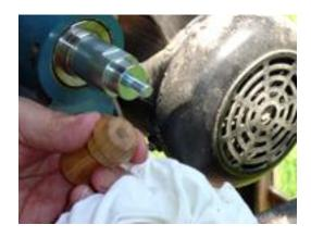
Screw the chrome cone stopper into the blank. The Bottle Stopper is Finished!
