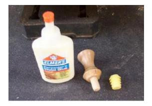
Apply a small amount of glue on the silicon stopper and mount on the wooden dowel. Let the glue dry and the stopper is finished.
