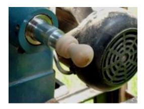
After the stopper is shaped, slow down the lathe speed to sand your stopper. I use 100, 150, 220, and 400 grit sandpaper.
