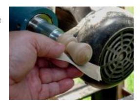
I use EEE-Ultra-Shine to finish the sanding process. This product is a wax base with fine grit that provides a fine smooth surface ready for finish.
