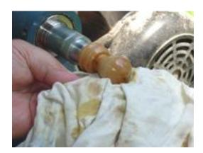
I then apply a coat of PPP wax. You apply the wax and then spin it at a high speed and polish it with a cloth.
