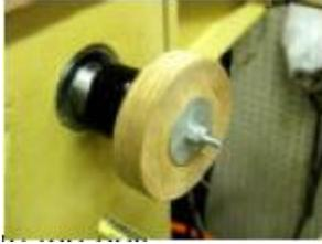
2) From the backside of the glue block, insert a 5/16" carriage bolt long enough to provide approximately 1" of threaded end exposed. Jam the carriage bolt so that it will not turn. Hold in place with a 5/16" nut. Make sure the bolt turns true on center. Use of a fender washer will help to stabilize the bolt.
