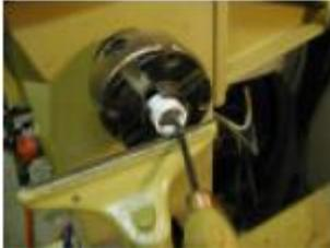
4) Remove the bushing, invert and re-insert into the glue block. The bearing can be installed and left in place to provide extra strength against the chucking force.
