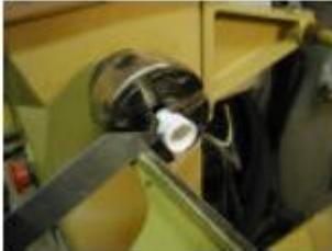
3) Carefully counter bore the ID for a press fit of the skate bearing. The depth of the counterbore should not be greater than the thickness of the bearing. Leave a shoulder for the bearing to seat against. Recommended tool is a mini bowl scraper made from a 3/16" Allen wrench using the shortened right angle leg for the cutter.
