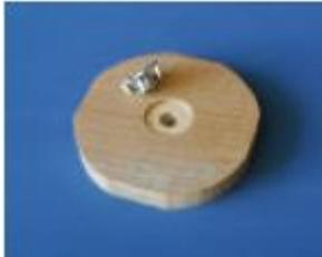
7) Press a T-Nut into each blank from the spot drilled side. Surface of the T-nut should be flush with the face of the blank.
