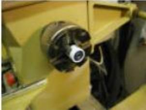
5) Turn the face of the bushing to establish an overall length of approximately 13/16".
