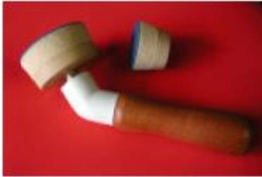
This is a process for building a rotating bowl sanding tool that is used for sanding the interior and exterior curved surfaces of turned bowls and similar projects. It is used by simply holding the sanding disk against the surface to be sanded while the bowl is rotating in the lathe. Spindle speed should be kept below 1000 RPM. The sanding disk rotation speed and direction will depend upon the angle and location of its contact with the surface.
