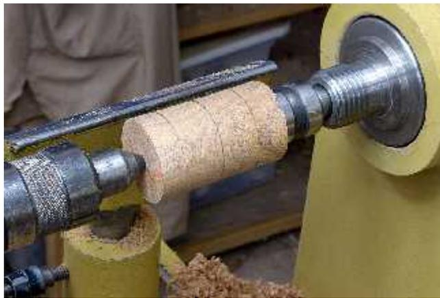
4. Turn the region on either side of the outer lines to about a  $5/8$  diameter inch 'spoke'. There's nothing critical about the diameter of the spoke.
