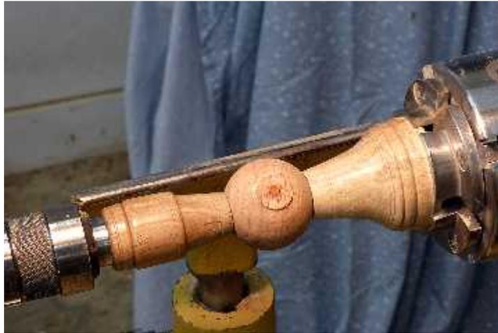
3. Turn off the remains of the spoke with a spindle gouge. Look for the shadow above and below the sphere; carefully turn the sphere until the shadow is gone. From this point on we'll be using a scraper to fine tune the shape.
