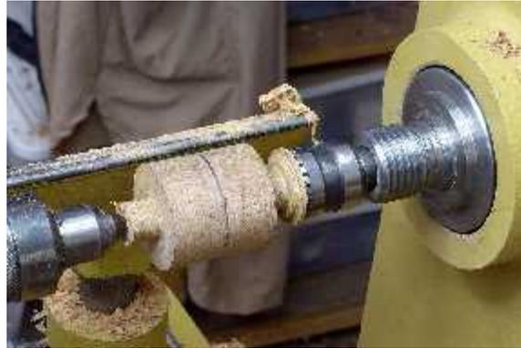
5. Round over the ends toward the spoke using a spindle or bowl gouge to an approximate sphere. Do not remove the center line in this step. For small spheres getting the sphere right at this point reduces the work of later steps, but isn't particularly critical. However for larger spheres it's important that the shape of the sphere be pretty close to right. Make a cardboard quarter round template to check your sphere's shape for bigger spheres (say, over 4 inches in diameter).
