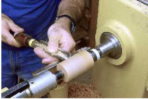
2. Mark a center line - the center line of the sphere; not necessary the center of the cylinder.
