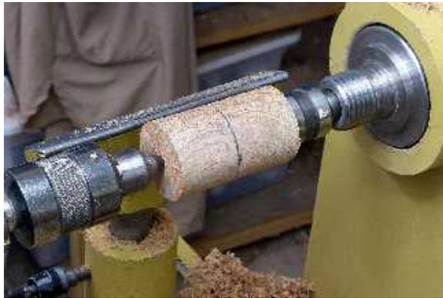
3. Mark 1/2 of the cylinder's diameter on each side of the centerline.
