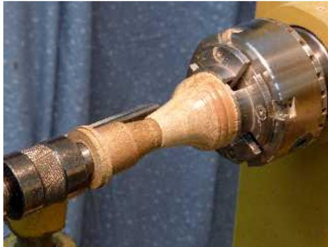
Shape the sides of the tailstock cup center.
