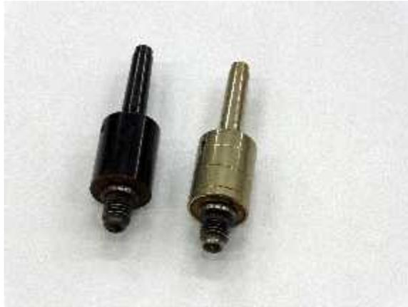
Turn a cylinder between centers and put an appropriate tennon on one end (dovetail or straight) to fit your four-jaw chuck.
