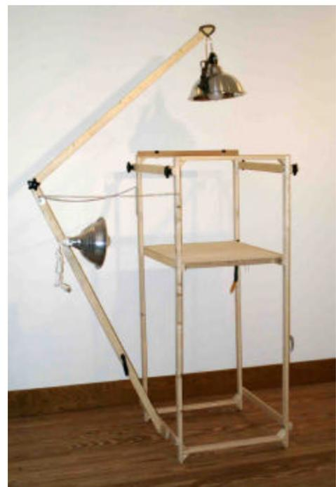
boom member is 52" long, and the upper boom member is 44". Light chain or cord is used to stabilize the boom near its joint. The cloth used for diffusion was the cheapest white cotton cloth I could find (2 yards at \$2 per yard). A couple of binder clips hold the seamless background in place.
