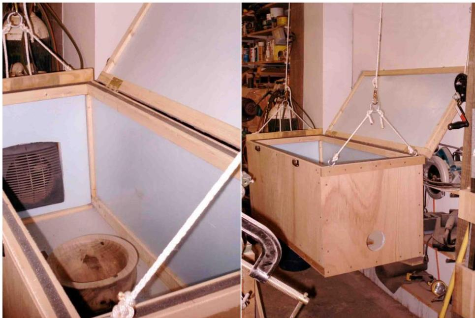
Look Drying box hanging from the ceiling with the lid open. Notice the winch in the upper right, and the 4" hole in the end of the box.
