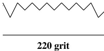
As you can see, the progressive sanding with higher grit paper yields smaller and smaller hills and valleys while reducing the thickness of the surface. This is the key to good surface preparation, i.e., progressive sanding to reduce the hills and valleys.
