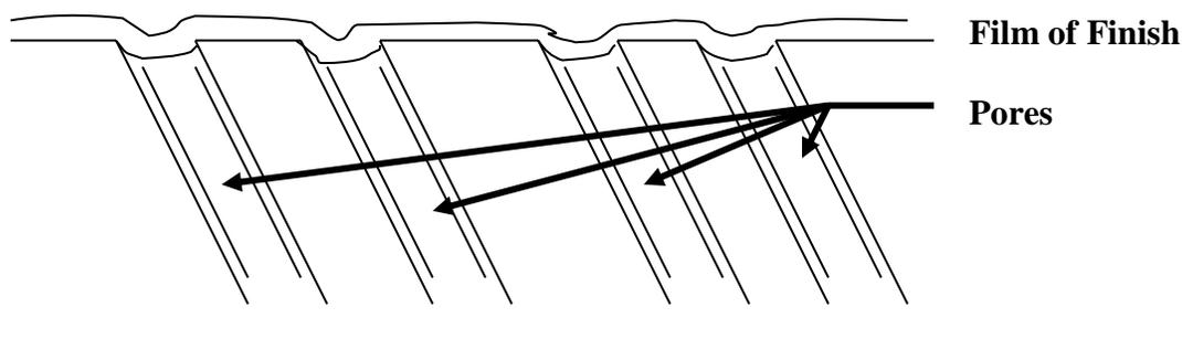
**Cross section of sagging pores at surface with film of finish**
